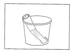
2. Place the contra angle in a paper cup with the connection end facing up and wait for 10 minutes.
