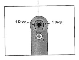
3. Put a drop of LS oil in each of the two points between the electrode cap and the contra head as indicated by the arrows in the illustration.
